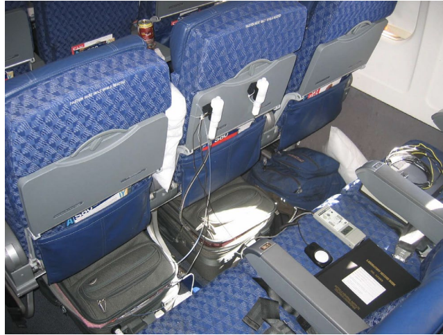
Figure 2-1. Onboard deployed samplers for environmental measurements [101].
